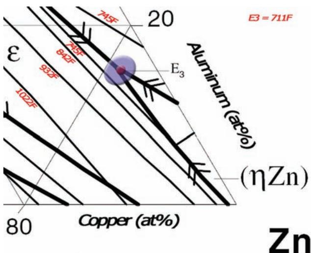
*Figure 2 – Ternary liquidus diagram of the Al/Cu/Zn system<sup>2</sup> (edited).<sup>#3</sup>*
