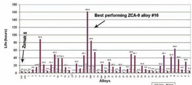
Figure 1 – ZCA-9 Results showing improved creep performance with test alloy #16.
