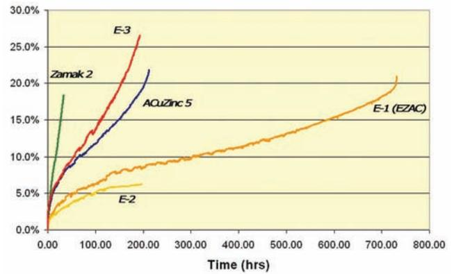
Figure 4 – Creep Curves for the alloys tested at MTU.
