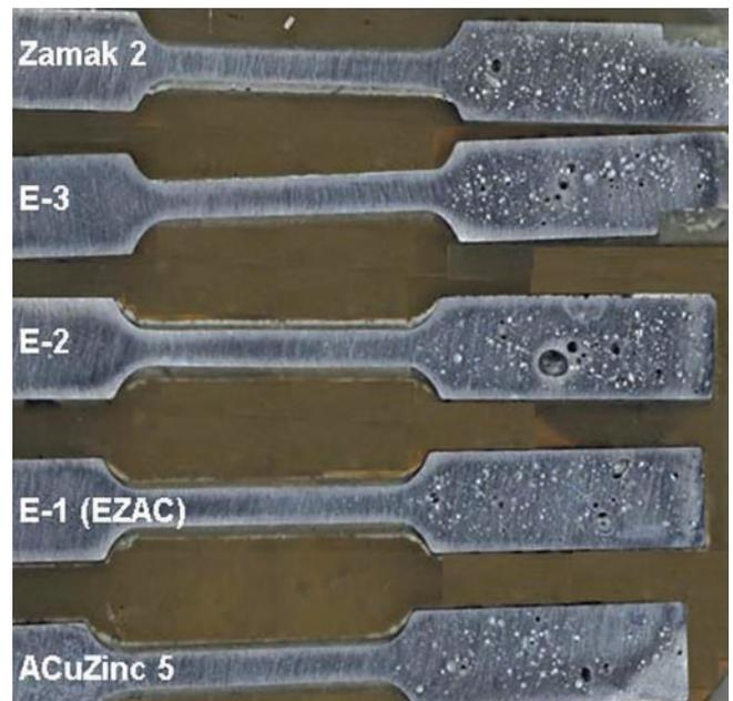
Figure 5 – Cross sectional view of the samples with resulting porosity content.
