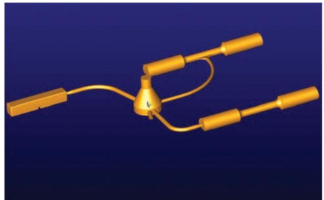
*Figure 3 – Tensile and impact specimens used for testing.*
