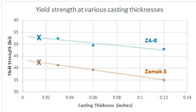
**Figure 5** - Data from ILZRO research program ZM-361 showing the relationship between casting thickness and yield strength (parameters were: water quench, 27 m/s gate velocity & 190° C die temperature).
