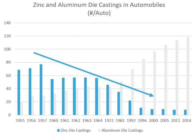
**Figure 2** - Zinc and Aluminum Die Castings in Automotive Applications. (Twarog, 2015)
