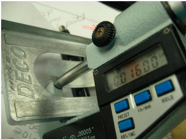
**Figure 1** - Thin Wall Card Holder - EZAC Alloy - 0.016" Thick.
