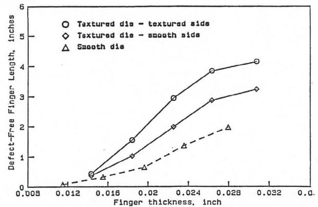
**Figure 4** - Castability Difference in Zamak 3 Die Castings Due to Texturing.
