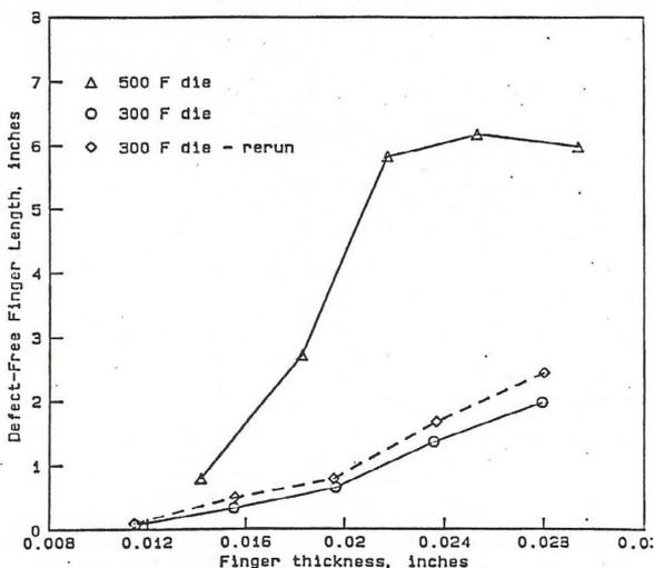
**Figure 3** - Castability Difference in Zamak 3 Die Castings Due to Die Temperature.
