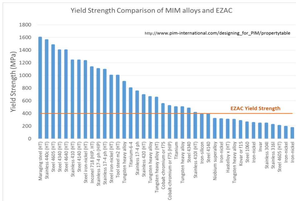
Figure 1: Yield strength comparison of common MIM alloys compared to EZAC.
