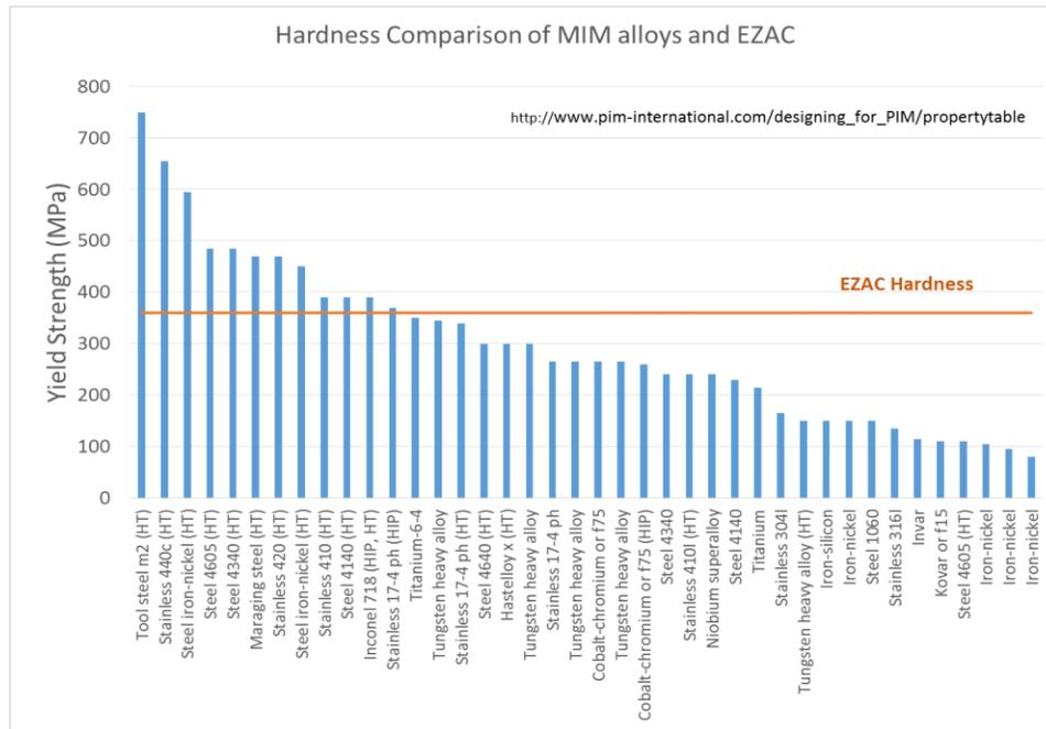
Figure 2: Hardness comparison of common MIM alloys compared to EZAC. (Note: EZAC's VHN hardness was converted from a Rockwell B value of 68.4)
