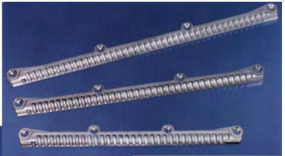
*Die-cast ACuZinc replaced P/M for these gear racks and provides greater wear resistance and strength. The racks are produced in lengths of 255 mm, 300 mm and 340 mm.*
