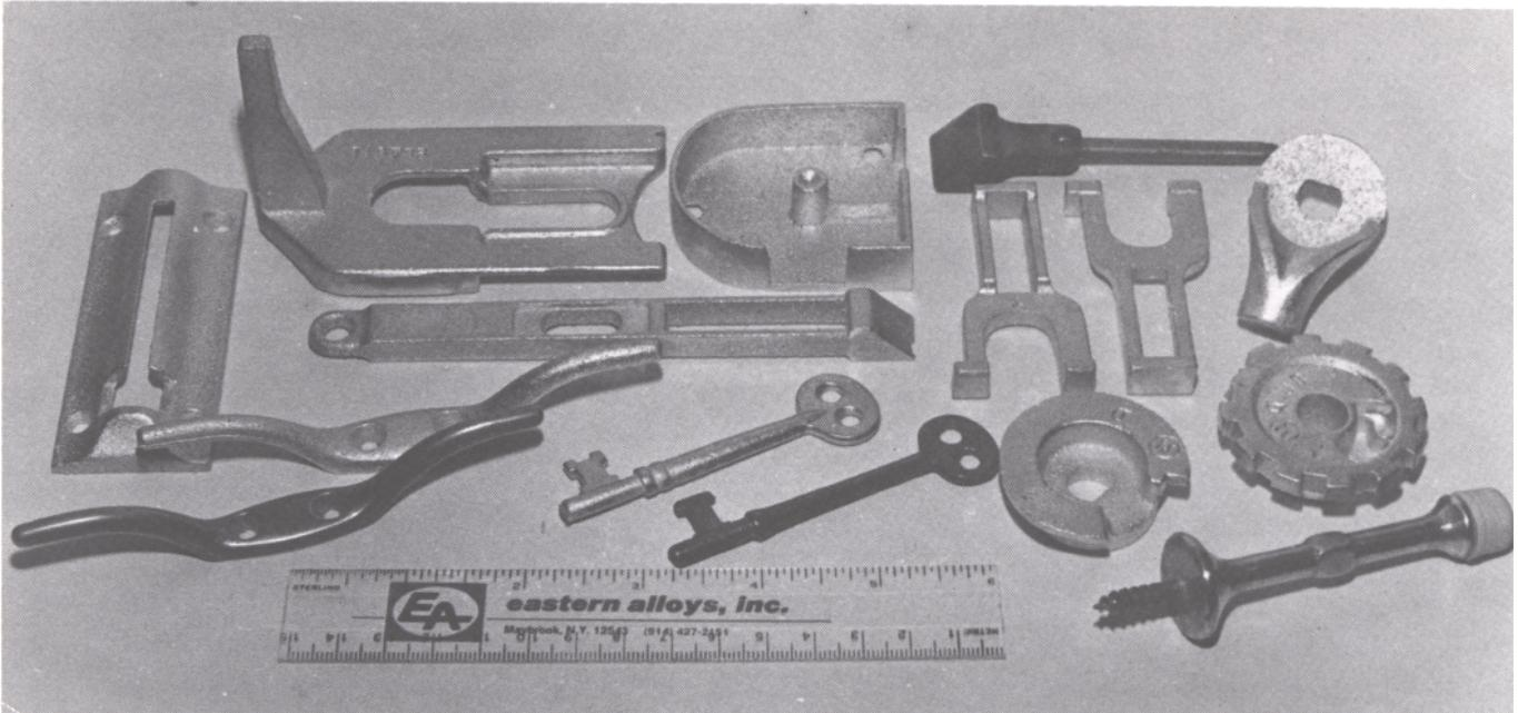
ZA-27 slashed costs and improved performance of these typical small parts formerly made of cast iron by Safe Hardware Corporation. Items shown include components of a door closer, internal lock units, chain bolt, door stop and skeleton keys.
