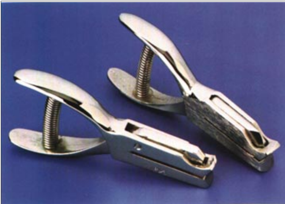
By converting to net-shape die casting, manufacturing operations were cut from 65 to 20 and manufacturing costs reduced 50 percent. The die-cast punch is shown on the left, the machined sand casting on the right.
