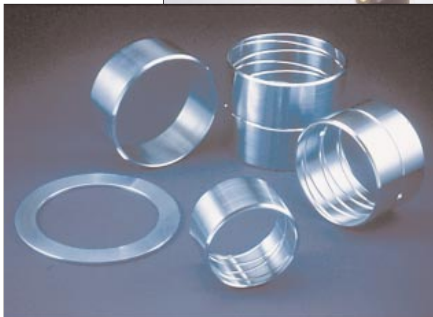
Champion's use of Concast ZA-12 bearings provides improved operating performance and cost-effective bearing properties for low-speed, high-load applications. Pictured here are bearings ranging in size from 3-1/2 in. I.D. x 4-3/4 in. O.D. x 1/8 in. thick (far left) to 3-1/2 in. I.D. x 3-3/4 in. O.D. x 3 in. long (upper right).
