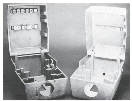
Rapidprint, Inc., switched their 25-lb. cast iron recorder housings (on Lt.) to ZA-12 zinc sand castings (on Rt.) and saved extensively on machining and finishing; ZA-12 was impact-tested over 300,000 cycles to assure years of rugged, dependable performance.
