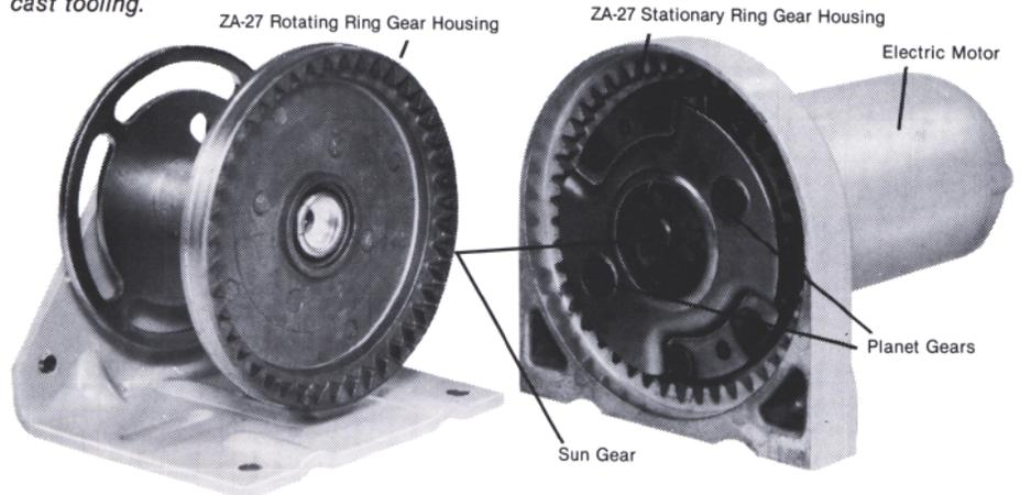
Efficient Superwinch design shows sun gear, driven by electric motor, and planet gears which revolve against 5-inch diameter die-cast ring gear housings (stationary and rotating). ZA-27 and aluminum parts are made in the same die-cast tools. ZA-27 components are used only in high-load winch modes where the superior strength and natural lubricity of ZA-27 is required.
