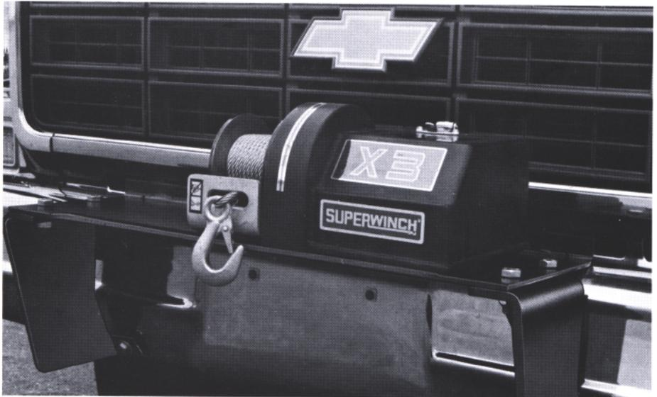
Recreational vehicle winches (Model X3 shown) manufactured by Superwinch, Inc., incorporate die-cast ZA-27 gear housings which were tested 2½ times stronger than 380 aluminum parts and allowed Superwinch to develop new high-load winches using existing die-cast tooling.
