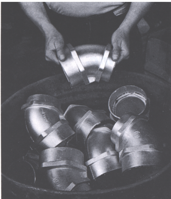
Large conduit elbow fittings are sandcast of Zn-12. Courtesy Lion Head Cast Products.
